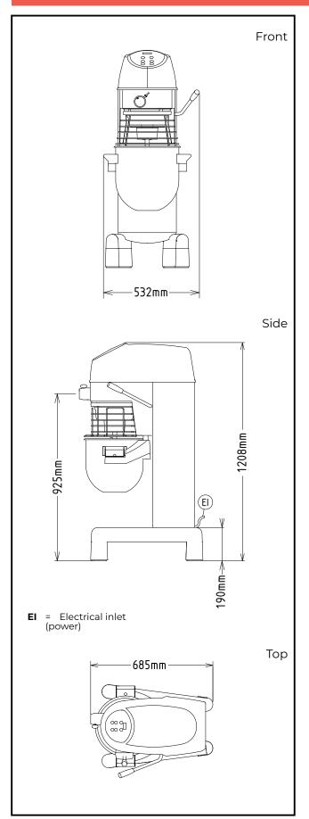
Electric Supply voltage: 200-240 V/1N ph/50/60 Hz Electrical power, max: 1.1 kW **Total Watts:** 1.1 kW Capacity: Performance (up to): 7 kg/Cycle Capacity: 30 litres Key Information: External dimensions, Width: 532 mm External dimensions, 685 mm Depth: External dimensions, Height: 1208 mm **Shipping weight:** 109 kg **Cold water paste:** 7 kg with Spiral hook **Egg whites:** 50 with Whisk
